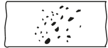
(a) Random Rounded Indications Typical concentration and size permitted in any 150 mm length of weld.
