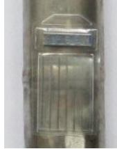
Figure 2: Wire type IQI
