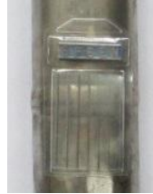
Figure 2: Wire type IQI
