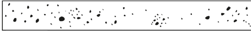
(a) Random Rounded Indications Typical concentration and size permitted in any 150 mm length of weld.
