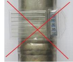
Figure 3: Not correct IQI placement
