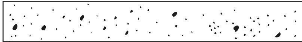
(a) Random Rounded Indications Typical concentration and size permitted in any 150 mm length of weld.
