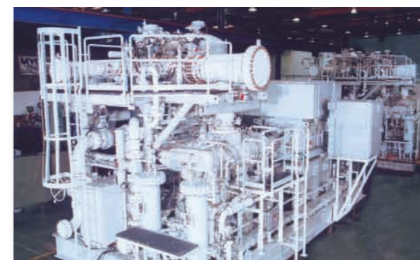
Offshore platform vapor recovery compressor
