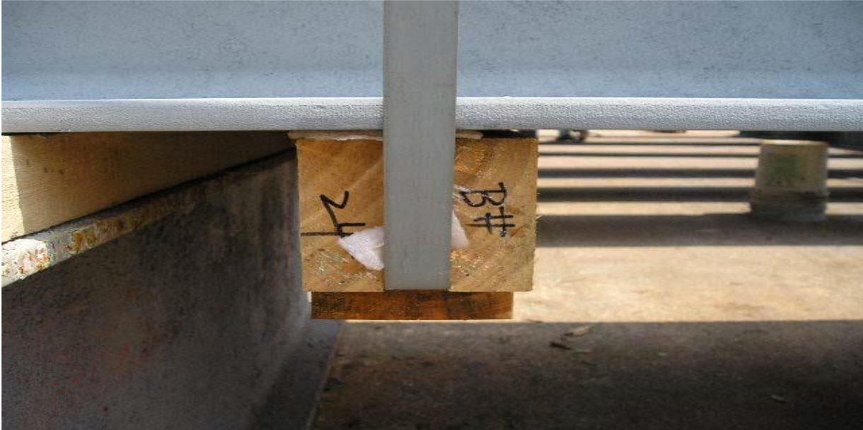
Figure 4. Using timber and belts in case of bundle type packing
