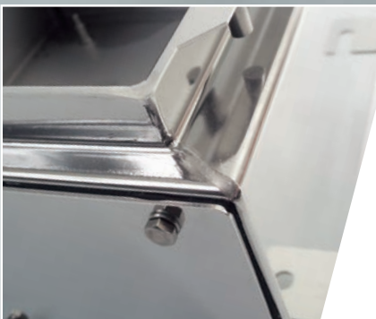
Detail of TIG welding of walls
